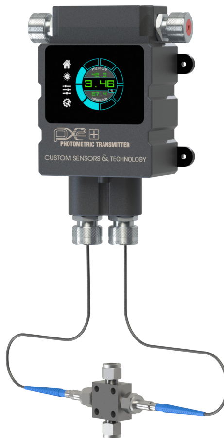
CST's Water in Ethanol Analyzer includes a PX2+ with (2) fiber optic cables and a cross flow cell with (2) optical interface couplers.
