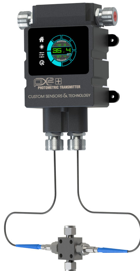
CST's Chlorine Analyzer includes a PX2+ with (2) fiber optic cables and a flow cell with (2) optical interface couplers
