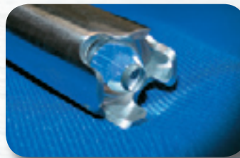
ATR crystal with guard for insitu measurement of asphaltenes in crude.
